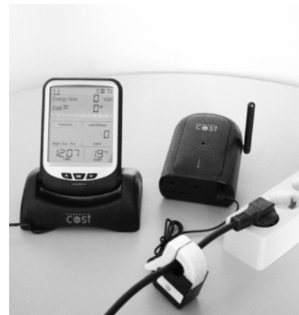
Fig. 2 components of the Current Cost power usage monitoring system
